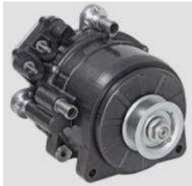
Continental's 5kW (max. 13kW) motor + inverter used by Volkswagen
