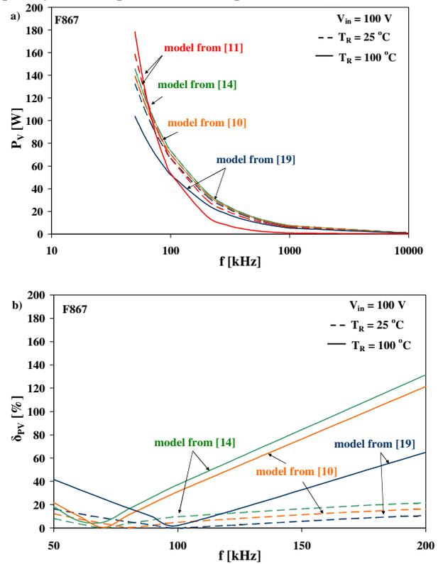
Fig. 7. The dependence of a) power losses in the ferrite core F867 and b) the power losses error on frequency for two values of the core temperature and  $V_{in} = 100$  V
