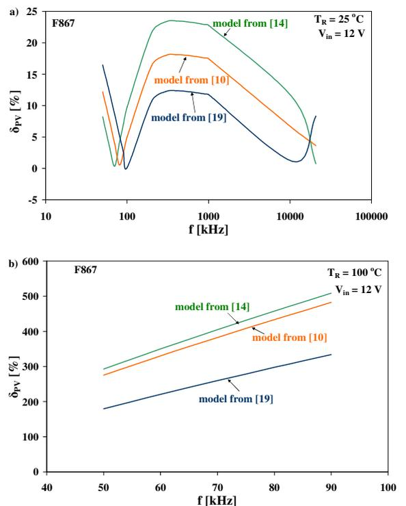
Fig. 8. The dependence of the power losses error in the ferromagnetic inductor core on frequency at  $V_{in} = 12$  V for the core temperature equal to a) 25 °C and b) 100 °C, respectively.
