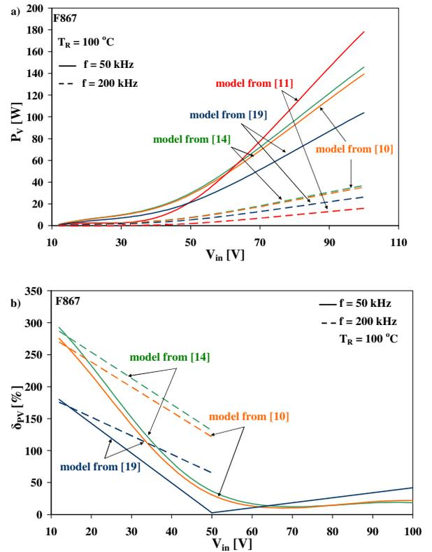
Fig. 5. The dependence of: a) power losses in the ferrite core and b) the calculation error of power losses on the input voltage at two values of control signal frequency equal to 50 and 200 kHz, respectively.
