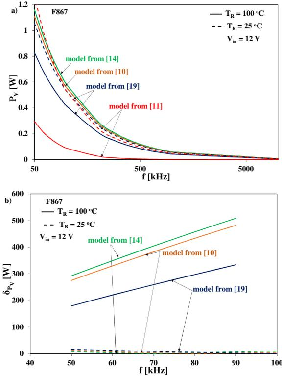
Fig. 6. The dependence of a) power losses in the ferrite core F867 and b) the error of power losses calculations on frequency at two values of the core temperature.
