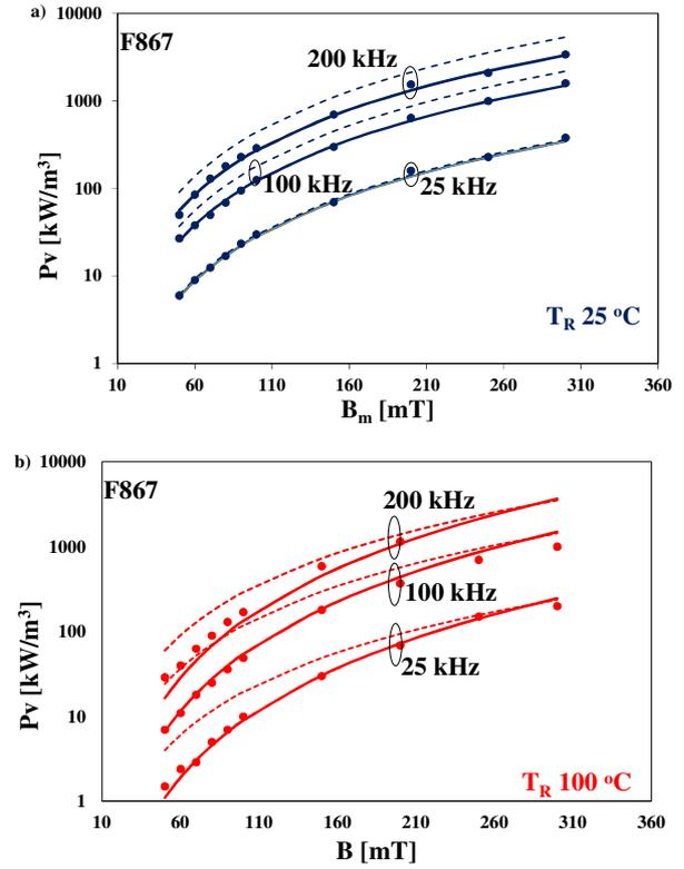
Fig. 2. The measured and calculated dependence of power losses per unit volume of F867 ferromagnetic material on the amplitude of magnetic flux density for temperature equal to: a) 25 °C, b) 100 °C
