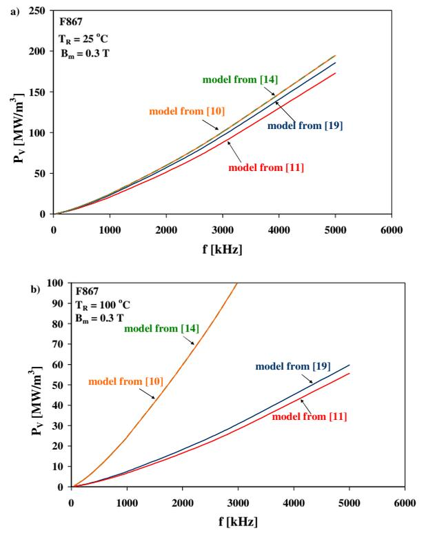
Fig.4. The dependence of power losses density in ferrite material F867 on frequency for two values of temperature equal to a) 25 and b) 100 °C, respectively.
