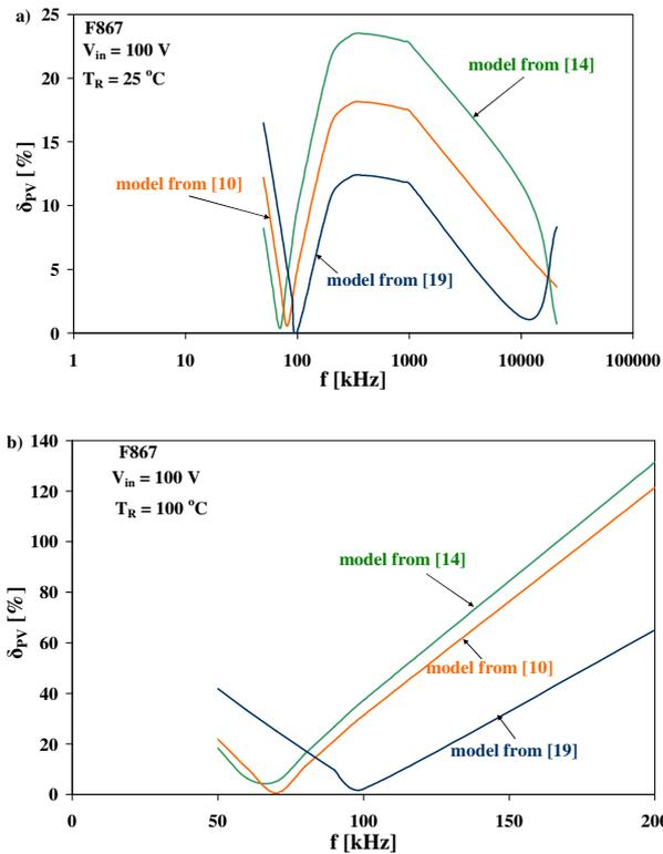
Fig. 9. The dependence of the power losses error in the ferromagnetic inductor core on frequency  $V_{in} = 100\text{ V}$  for the core temperature equal to a)  $25^\circ\text{C}$  and b)  $100^\circ\text{C}$ , respectively.
