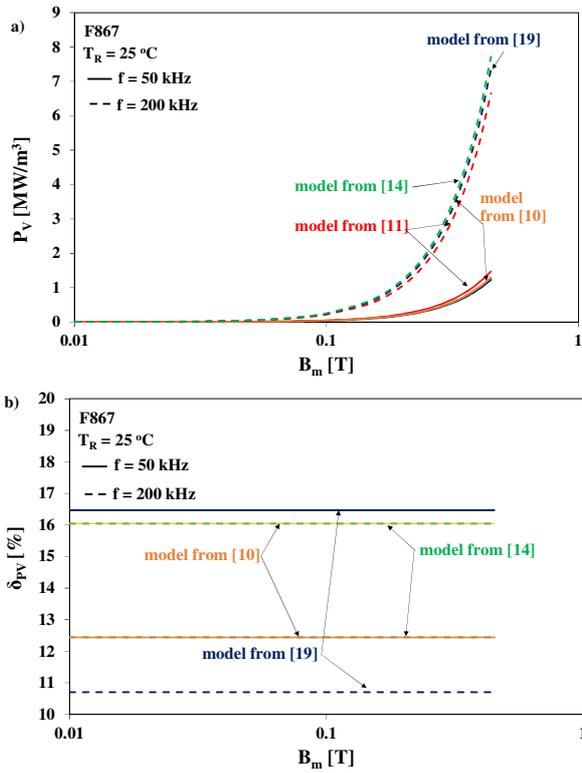
Fig.3. The calculated dependence of: a) power losses in ferrite material F867 and b) calculation error on the amplitude of magnetic flux density at frequency equal to 50 and 200 kHz, respectively.
