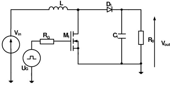
Fig.1. The diagram of the boost converter
