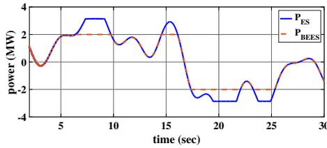
Fig. 12: Active power support from BESS
