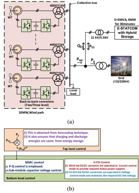
Fig. 1: (a) Grid connected WEGS with H-ESS based E-STATCOM, (b) Overview of E-STATCOM control
