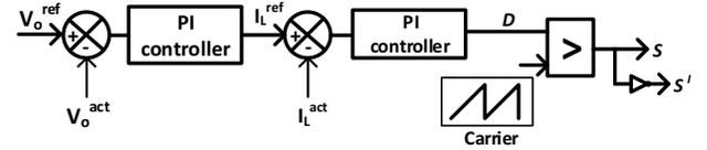
Fig. 6: Control block diagram of supercapacitor fed DC-DC converter
