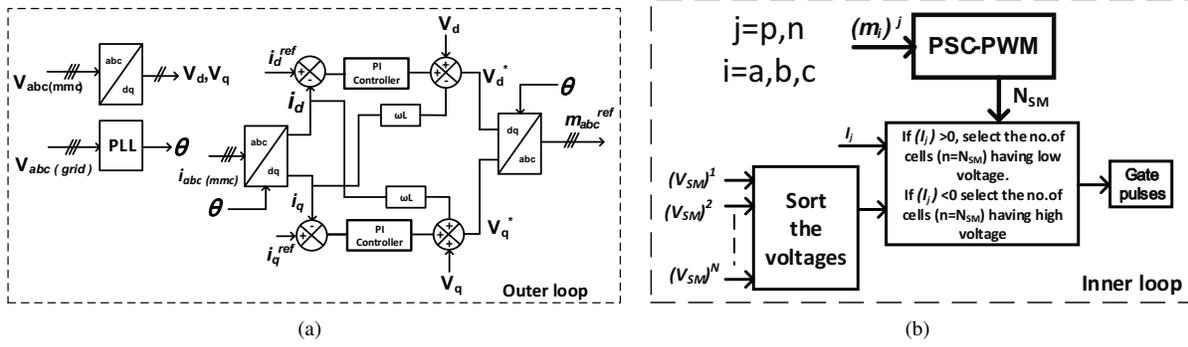
Fig. 4: (a) Outerloop control of MMC for active and reactive power support, (b) Sub-module capacitor voltage balance algorithm
