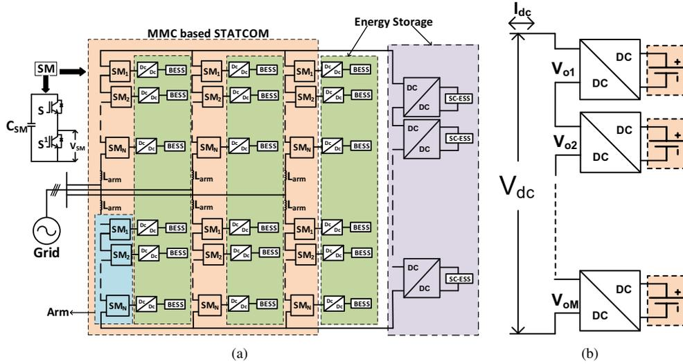
Fig. 2: (a) MMC based Hybrid Energy Storage system, (b) Cascaded DC-DC converter connected at DC link
