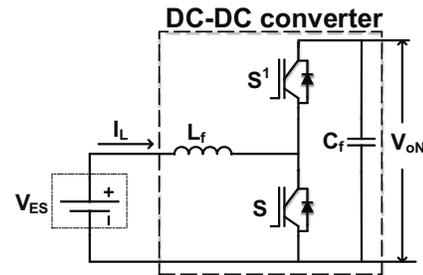
Fig. 3: Bi-directional DC-DC converter for ES integration
