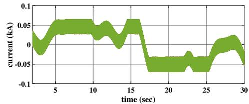
Fig. 11: Actual and reference currents drawn from BESS at the sub-module
