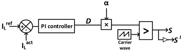
Fig. 5: Control block diagram of BESS fed DC-DC converter
