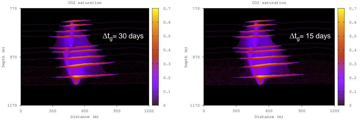
These two very similar figures show that it is enough to use a formation time step  $\Delta t_g$  of 30 days to update the parameters (k,  $\phi$ ) in the flow simulator.
