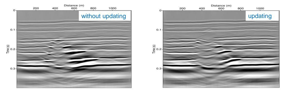
When the simulation parameters are updated (right figure) the CO2 plume induces the pushdown effect in a wider region in the horizontal direction, and moves faster in the vertical direction as compared with the left figure, obtained without updating parameters
