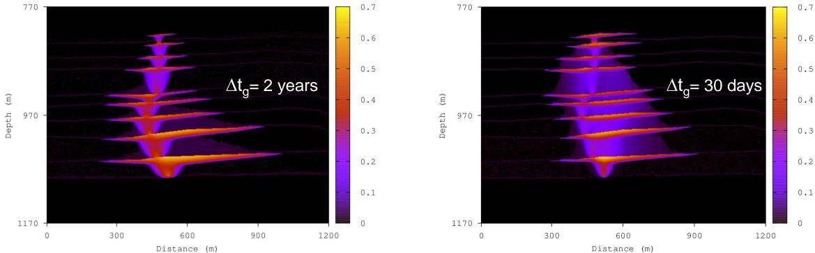
The left figure, obtained without updating flow parameters, shows very well defined chimneys and accumulations below the mudstone layers. The right figure, computed updating every 30 days, displays a less defined chimney, thinner accumulations and more extended CO2 zones between mudstone layers.
