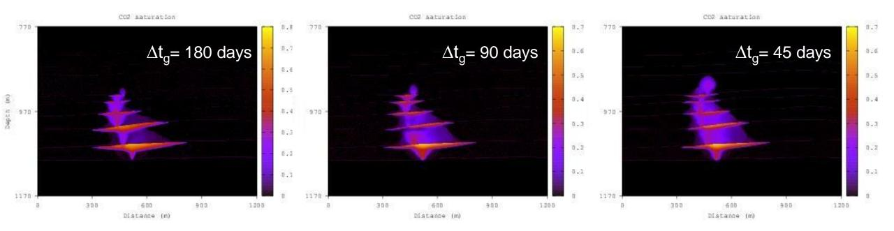
Because  $k_z$  is saturation dependent, the CO2 plume is seen to move upwards faster when the petrophysical properties are updated more frequently, i.e., as  $\Delta t_a$  is reduced
