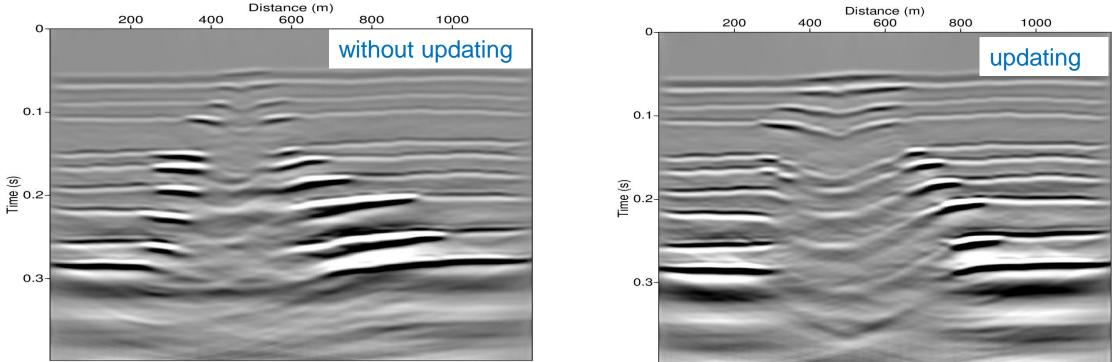
Again, the CO2 plume moves faster in the vertical direction and induces the pushdown effect in a wider region in the horizontal direction when the petrophysical and seismic properties are updated
