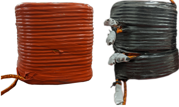
Fig. 2. Conventional winding arrangement (red) and triple fold-back winding arrangements (black).
